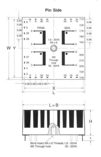
Dimensions in mm. Electrical measurements @20'C ambient temperature.
