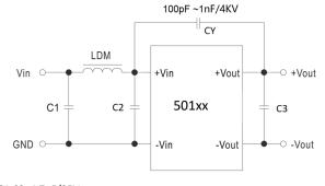
C1: 10uF/16V@5Vdc Vin; : 2.2uF/25V@12Vdc Vin; : 1.0uF/25V@24Vdc Vin;
