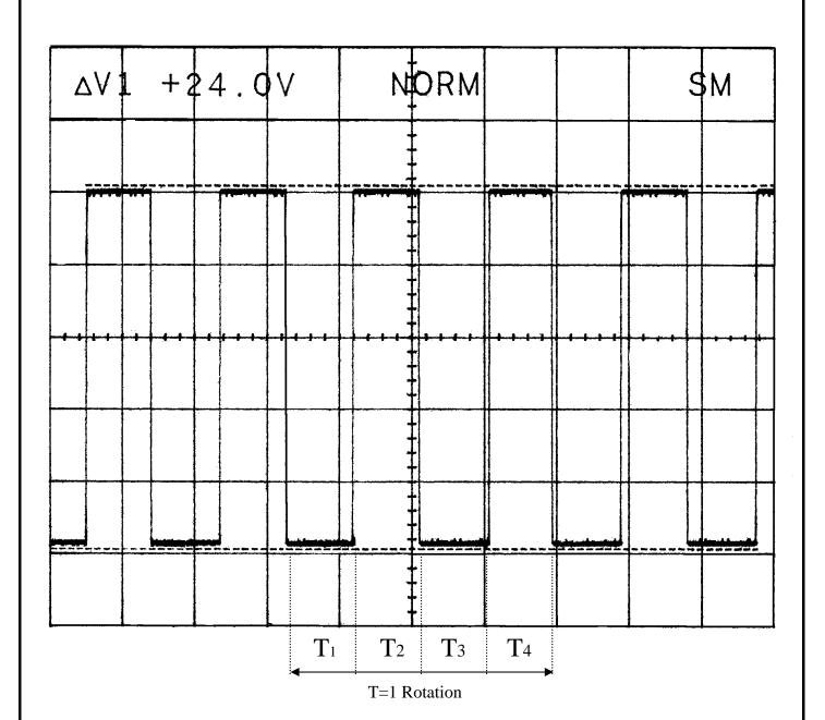
T=T1+T2+T3+T4 =(1 Rotation) T1=T2=T3=T4= $\frac{60}{4 \times \text{rpm}}$
