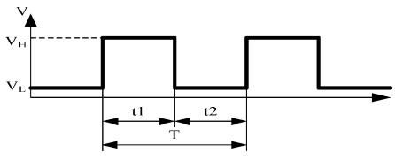
$$T = \frac{1}{|f|_{\text{PWM}}} = \text{t1} + \text{t2(sec)} \quad . \label{eq:T_pwm}$$
