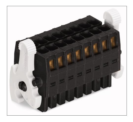
Printview: Female connector; with ejectors; 5x2-pole; pin spacing 3.5 mm / 0.138 in; 100% protected against mismating; 2 rows; with coding fingers to be cut off - Item No.: 713-1105/037-000
