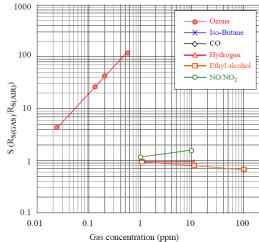
Fig 3. Sensitivity characteristics
