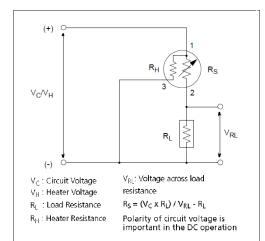
Fig 2. Standard circuit
