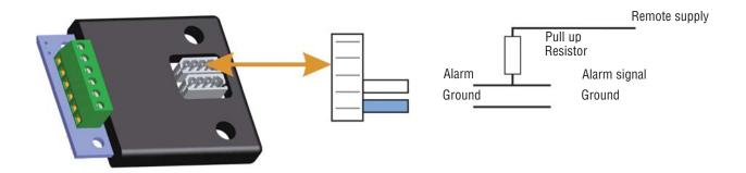
The alarm output cable should only be connected to the upper of the two connectors shown above. The other is reserved for future expansion.
