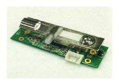
IR-93 can accurately detect carbon dioxide between 400 to 4,000 ppm.
