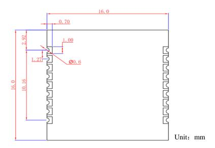
Pic2. Module Dimension Diagram
