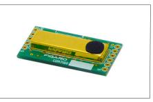
measurement possible. Every module is individually calibrated and is provided with both a UART and I2C digital interface. The CDM7160 module is designed for simple integration into a user's products. It can be used in a wide range of applications such as ventilation controls for the improvement of energy savings and to assure a good indoor climate.
