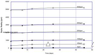
Fig. 8-1 - Durability of CDM7160 to high temperature (60°C)
