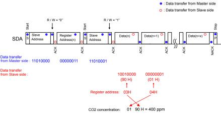
Fig. 12 - Data transfer sequence for random Read command
