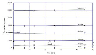
Fig. 8-2 - Durability of CDM7160 to low temperature (-10°C)
