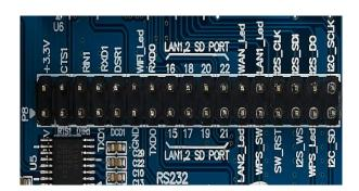
Almost all the pins of WizFi630S can be connected via the external connector.
