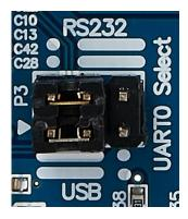
WizFi630S-EVB supports the UARTO Interface via 9pin D-sub(DB9) or micro USB.
