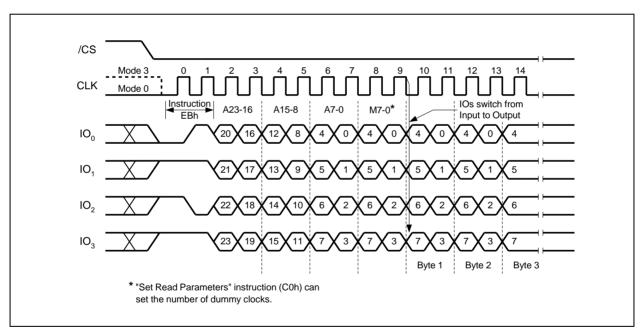
Figure 27d. Fast Read Quad I/O Instruction (Initial instruction or previous M5-4≠10, QPI Mode)
