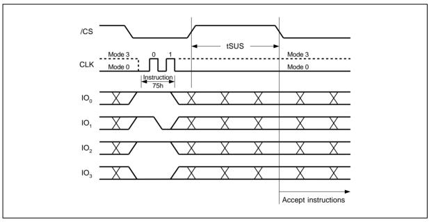
Figure 35b. Erase/Program Suspend Instruction (QPI Mode)
