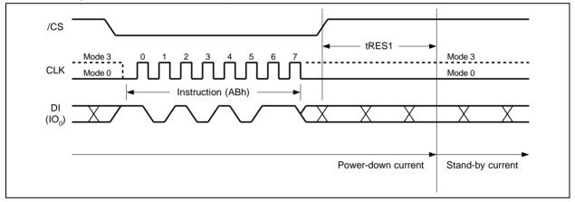
Figure 38a. Release Power-down Instruction (SPI Mode) /CS Mode 3 Mode 0 Mode 0 Instruction ABh Power-down current Stand-by current
