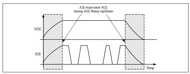
Figure 58b. Power-up, Power-Down Requirement
