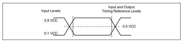
Figure 59. AC Measurement I/O Waveform
