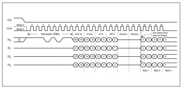
Figure 24a. Fast Read Quad I/O Instruction (Initial instruction or previous M5-4≠10, SPI Mode)
