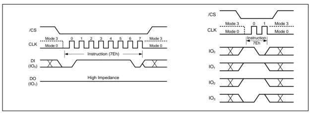
Figure 56. Global Block Lock Instruction for SPI Mode (left) or QPI Mode (right)
