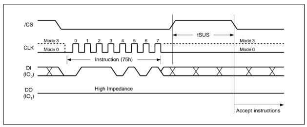
Figure 35a. Erase/Program Suspend Instruction (SPI Mode)
