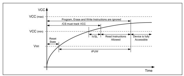
Figure 58a. Power-up Timing and Voltage Levels
