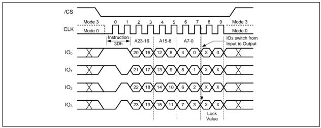
Figure 55b. Read Block Lock Instruction (QPI Mode)
