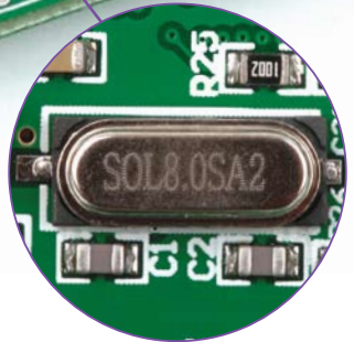
Figure 5-1: External crystal oscillator (X1)
