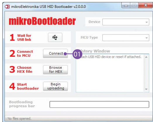
Figure 3-2: USB HID mikroBootloader window
