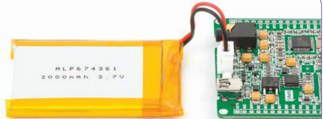
Figure 1-2: Connecting Li-Polymer battery
