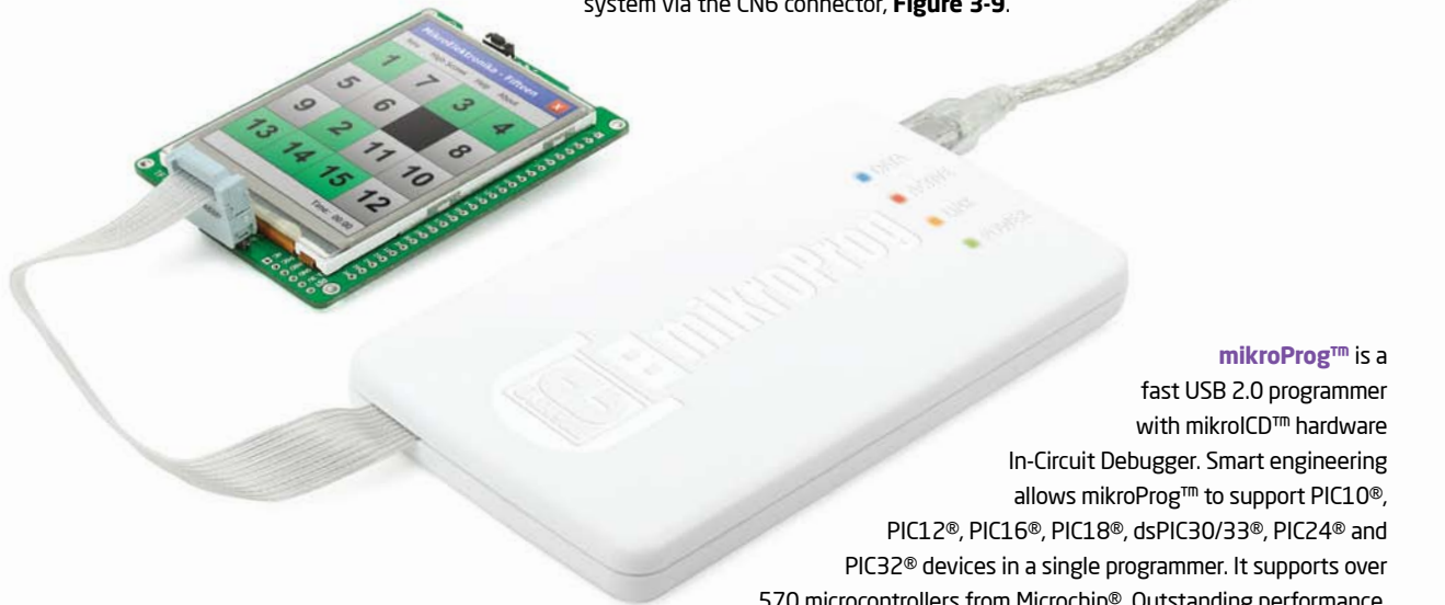
Figure 3-9: Connecting mikroProg™ to mikroMedia™
