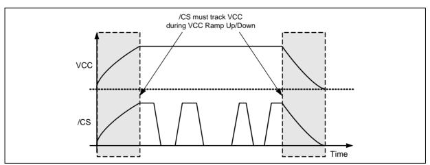
Figure 58b. Power-up, Power-Down Requirement
