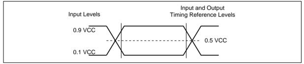
Figure 59. AC Measurement I/O Waveform
