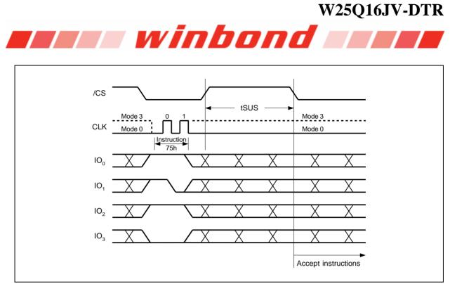
Figure 35b. Erase/Program Suspend Instruction (QPI Mode)
