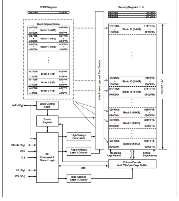
Figure 2. W25Q16JV Serial Flash Memory Block Diagram
