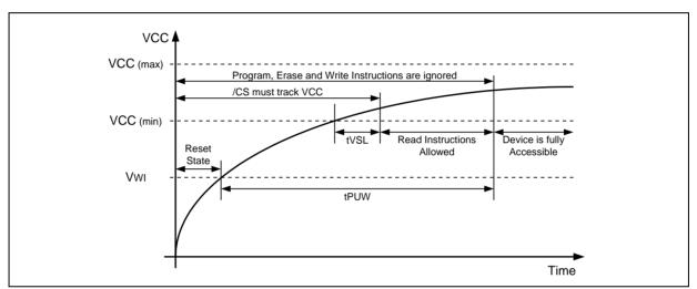
Figure 58a. Power-up Timing and Voltage Levels
