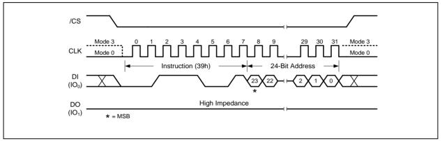
Figure 54a. Individual Block Unlock Instruction (SPI Mode)
