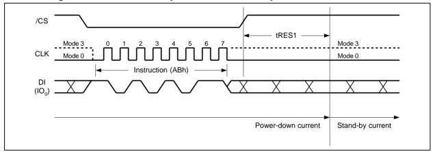
Figure 38a. Release Power-down Instruction (SPI Mode)
