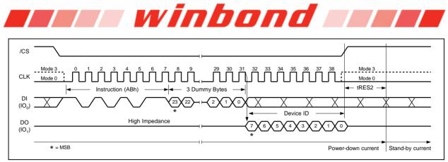
Figure 38c. Release Power-down / Device ID Instruction (SPI Mode)
