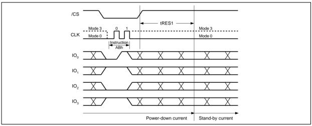
Figure 38b. Release Power-down Instruction (QPI Mode)
