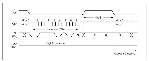
Figure 35a. Erase/Program Suspend Instruction (SPI Mode)
