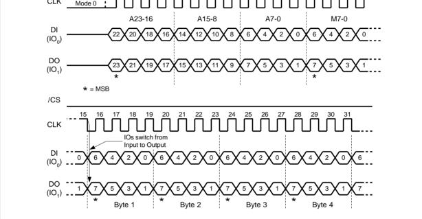
Figure 22b. Fast Read Dual I/O Instruction (Previous instruction set M5-4 = 10, SPI Mode only)
