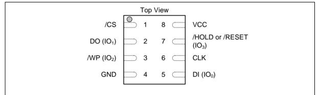
Figure 1b. W25Q16JV Pad Assignments, 8-pad WSON 6x5-mm, USON 2X3-mm/4x3-mm (Package Code ZP, UX, UU)
