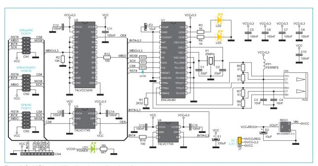
Figure 3: Serial Ethernet additional board connection schematic
