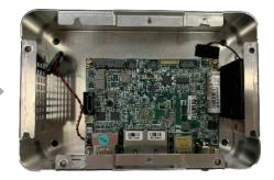
**Step 8: :** Reattach nut and washer to DC jack.
