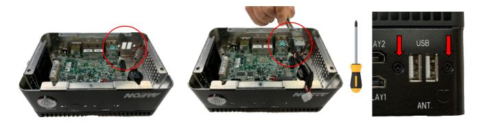
Step 13: Attach SATA cable to CN7 and SATA Power cable to CN9. DO NOT attach to storage device at this time.
