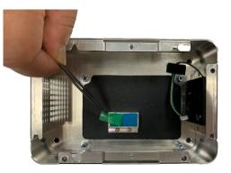
Step 5: Remove nut and washer from DC jack. Connect fan power cable to board (CN15).
