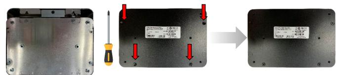
**Step 16:** VESA Mount (Requires VESA mounting kit). To use a VESA mount, attach two VESA mount screws to the bottom of the system as shown. Make sure the VESA bracket is attached to mounting surface with arrow pointing up. Slide the system into the mount as shown. (Figure is for demonstration purposes).
