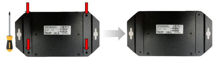
**Step 18:** Dual COM Port installation (optional). Remove I/O punchouts from front of system. Remove the retainer screws from each port connector, four in total.
