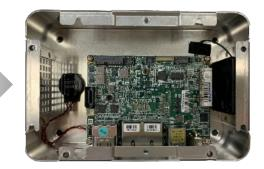
**Step10:** Thread the power button cable through the hole for the power button. Button should line up with notch at the top of the hole. Plug the cable into the front panel connector (CN3), then gently push the power button in until it is secure (you will hear a 'click').
