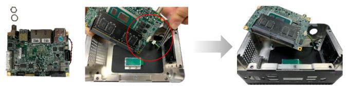
**Step 6:** Insert the PICO-WHU4 board into the chassis assembly with the processor side toward the heatsink. DO NOT place the CMOS battery between the board and thermal assembly. Make sure the processor is contacting the thermal padding and the holes line up with board and mounting points.
