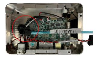
**Step 14:** Attach 2.5" drive to drive bracket, secure with four screws as shown. Note orientation with arrow. Attach SATA and SATA Power cables to drive, then attach the assembly to the system (Note: arrow points towards fan).
