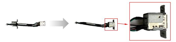
**Step 12:** Insert bracket into system with opening pointed towards heatsink (check image below for alignment). Secure to I/O panel with two black screws as shown. Connect cable to USB 2.0 port connector (CN19).
