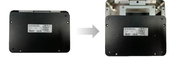
**Step 2:** Remove the two screws securing the 2.5" drive bracket. Remove the bracket and set aside. Using a tool, remove the USB 2.0 port punchouts if you haven't already done so.
