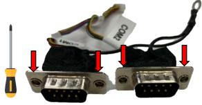
**Step 19:** Line up the COM ports with the correct holes. Check the attached labels to ensure the ports are mounted to the matching labeled I/O hole. Secure with retainer screws.
