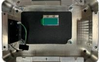
**Step 3:** On the processor side of the PICO-WHU4 board, install the memory RAM module. Insert at an angle (~30°) and then gently press down until it is secured in place.
