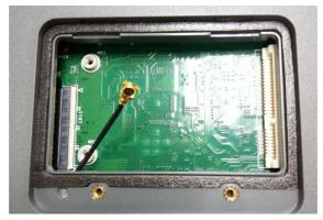
4. Slide the LTE module into the socket
