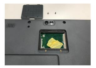
3. Remove the tape and pull up the antenna cable
