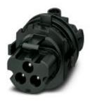
Circular connectors (cable-side), Range of articles: PRC, Contact insert, housing material: PPE, color: black, number of positions: 3, min. conductor cross section: 1.5 mm², max. conductor cross section: 6 mm², nom. voltage: 690 V AC, rated current: 35 A, Connection method: Screw connection, Type of contact: Pin
