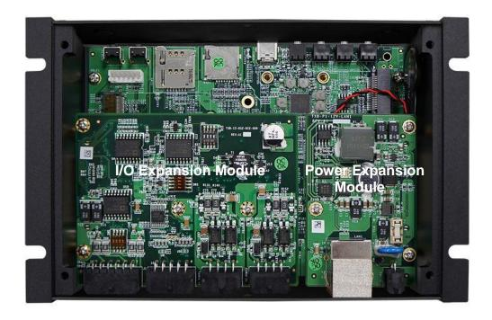
NOTE: Internal connectors and switches are accessible only after removing the I/O Expansion and Power Expansion modules.
