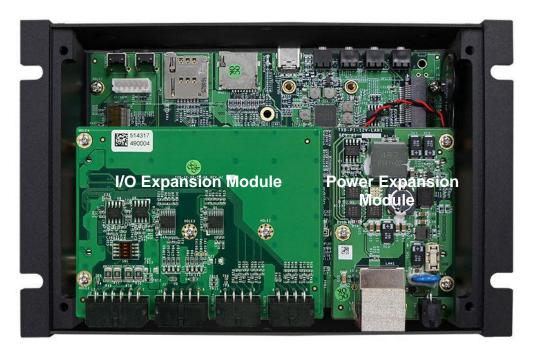
NOTE: Internal connectors and switches are accessible only after removing the I/O Expansion and Power Expansion modules.
