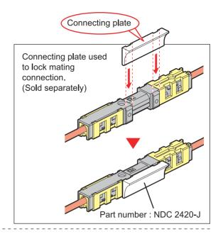
2 Link the connectors together for multi pole connection.
