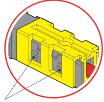
Confirm that it is correctly locked. (Two locking mechanisms on both sides.)
