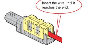
2 Making insulation displacement connection.
