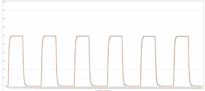
The test results show that the repeatability error range is <5ppm (100ppm ± 1% of full scale is the normal range);
