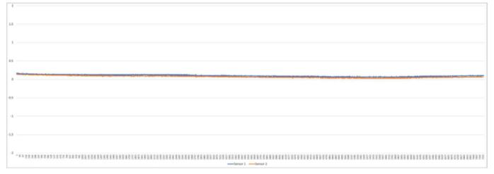
Test results: 12 hours clean air test, zero drift <0.3ppm (0-1ppm is the normal zero fluctuation range);
