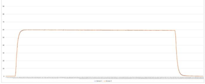
Test result: 2 hours ventilation, range drift <5ppm;
