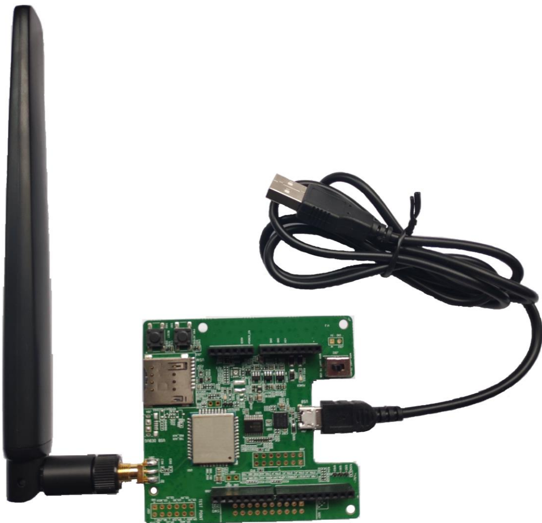
Figure 14: BC65-TE-B Kit Assembly
