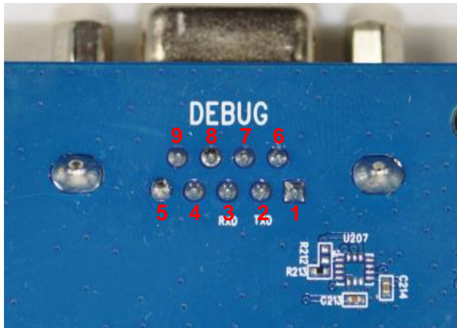
Figure 25: Pin Assignment of Debug UART Port (J604)
