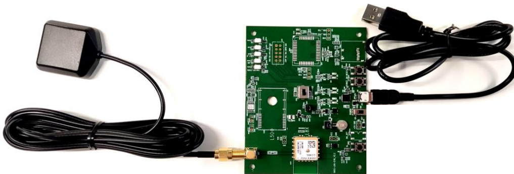
Figure 2: EVB and Accessories Assembly
