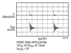
Figure 3. Burst Mode Operation
