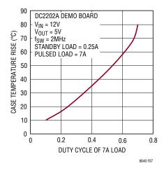
Figure 7. Case Temperature Rise vs 7A Pulsed Load
