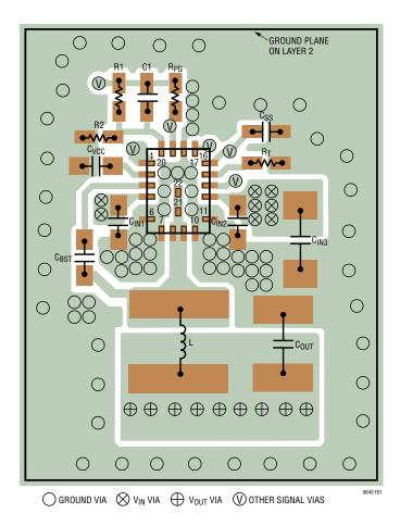
Figure 1. Recommended PCB Layout for the LT8640/LT8640-1
