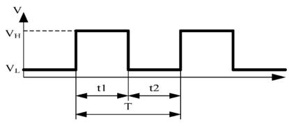
$$T = \frac{1}{f_{\text{PWM}}} = t1 + t2(\text{sec}) \quad . \label{eq:T_pwm}$$
