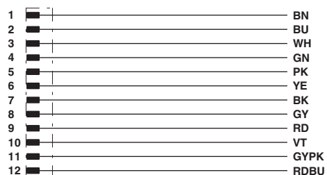
Contact assignment of the M12 plug
