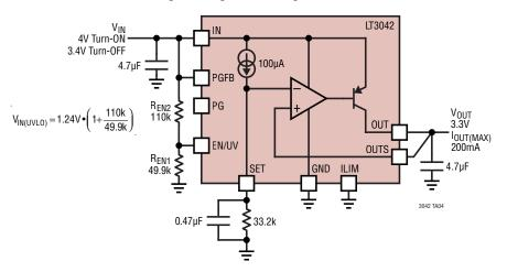
Programming Undervoltage Lockout
