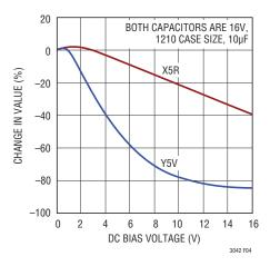
Figure 4. Ceramic Capacitor DC Bias Characteristics
