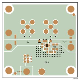
Figure 8. Example DFN Layout
