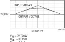
$R_{SET} = 33.2 k\Omega$   $C_{OUT} = 4.7 \mu F$   $C_{SET} = 0.47 \mu F$  $R_L = 16.5 \Omega$
