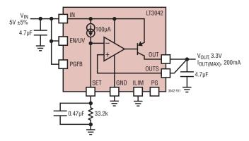
Figure 1. Basic Adjustable Regulator
