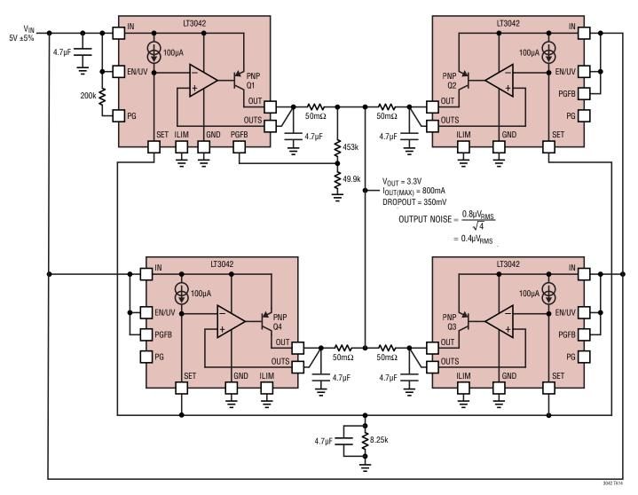
Paralleling Multiple LT3042s for Higher Output Current
