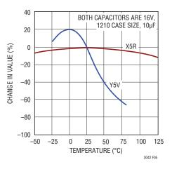
Figure 5. Ceramic Capacitor Temperature Characteristics
