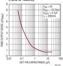
Integrated RMS Output Noise (10Hz to 100kHz)
