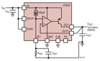
Figure 3.  $C_{\text{OUT}}$  and  $C_{\text{SET}}$  Connections for Stability
