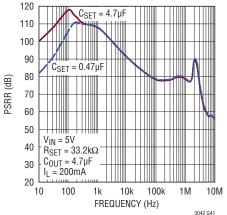
Power Supply Ripple Rejection
