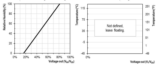
**Figure 7:** Relationship between the analog voltage output and the measured relative humidity corresponding to equation 9 for the SHT40I-KD1B.
