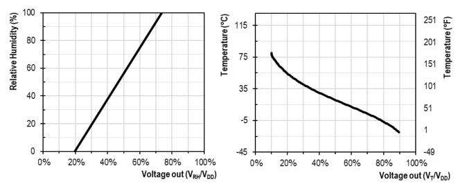
**Figure 5:** Relationship between the analog voltage output and the measured relative humidity and temperature corresponding to equations 4 and tabulated values in (5) for the SHT40I-ID1B.
