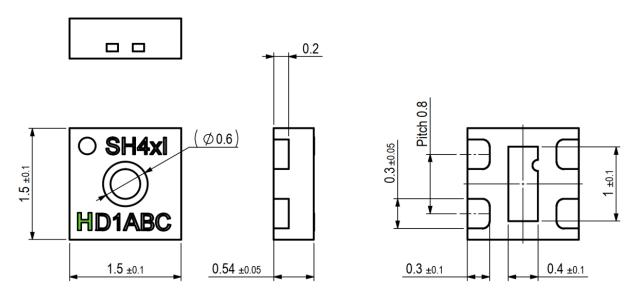
**Figure 8:** Dimensional drawing of SHT40I analog including package tolerances (units mm), where the H (here highlighted in green for better identification) serves as indicator for the standard analog interface. Other letters alphabetically after the letter H, indicate other versions of the analog interface, as detailed in **Table 11** and described in section 4.4.
