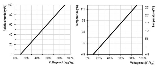
**Figure 4:** Relationship between the analog voltage output and the measured relative humidity and temperature corresponding to equations 1, 2, and 3 for the SHT40I-**H**D1B.
