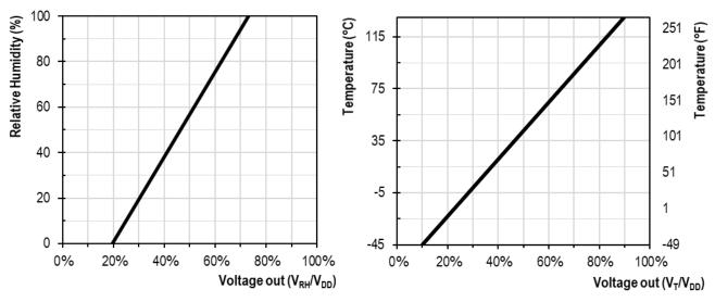
**Figure 6:** Relationship between the analog voltage output and the measured relative humidity and temperature corresponding to equations 6, 7, and 8 for the SHT40I-JD1B.
