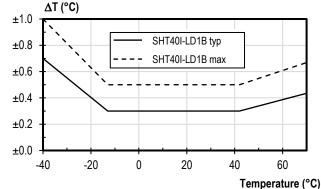
**Figure 2:** SHT40I analog (output characteristics H,I,J, K, *vide infra*) typical and maximal temperature accuracy, where model SHT40I-ID1B is only specified between -20°C and +80°C.
