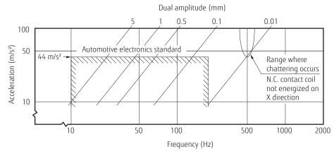
Frequency: 10 ~ 2000Hz Acceleration: 100m/s² max. Direction of vibration: See diagram below Detection level: Chatter >1ms
