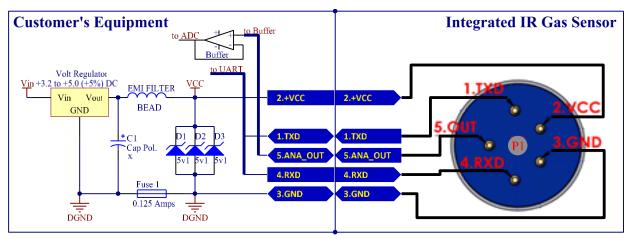
Fig. 1 -Example schematic for Interfacing Integrated IR (INIR)
