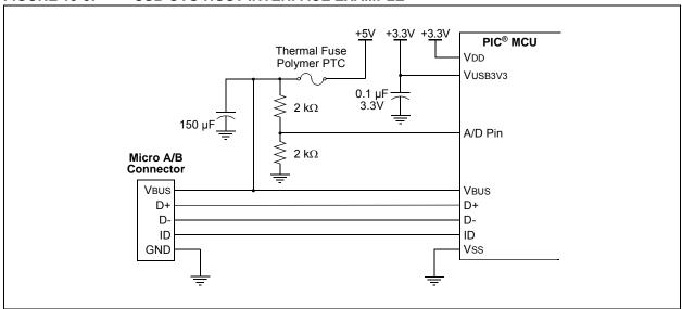
FIGURE 19-6: USB OTG INTERFACE EXAMPLE
