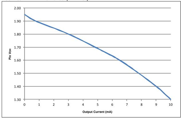
FIGURE 38-28: IOL vs. PIN VOL (VDD = 3.6V)
