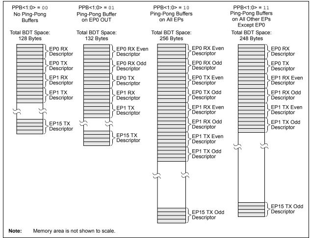
BDs have a fixed relationship to a particular endpoint, depending on the buffering configuration. Table 19-2 provides the mapping of BDs to endpoints. This relationship also means that gaps may occur in the BDT if endpoints are not enabled contiguously. This, theoretically, means that the BDs for disabled endpoints could be used as buffer space. In practice, users should avoid using such spaces in the BDT unless a method of validating BD addresses is implemented.
