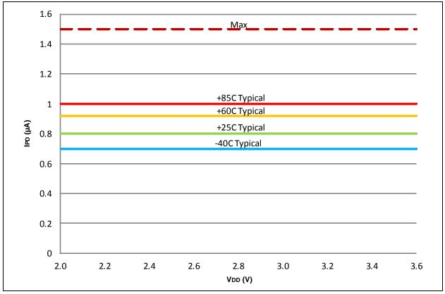
FIGURE 38-21: HLVD DELTA IPD vs. VDD
