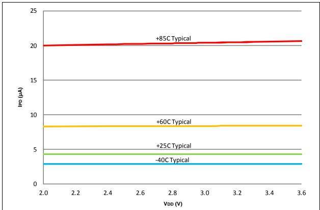
FIGURE 38-15: LOW-VOLTAGE SLEEP IPD (+85°C/-60°C) vs. VDD
