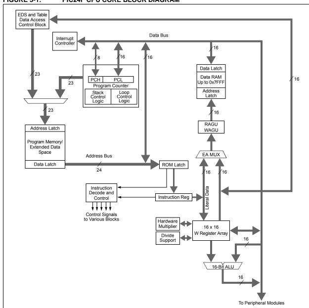
FIGURE 3-1: PIC24F CPU CORE BLOCK DIAGRAM
