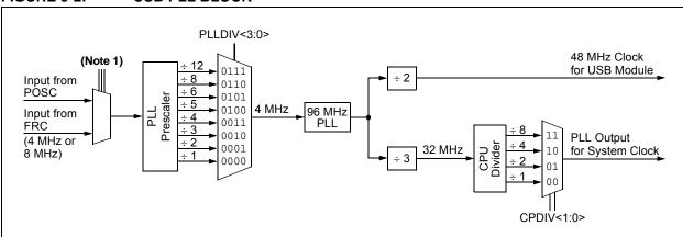
Note 1: This MUX is controlled by the COSC<2:0> bits when running from the PLL or the NOSC<2:0> bits when preparing to switch to the PLL.
