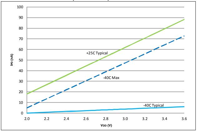
FIGURE 38-19: BOR DELTA IPD vs. VDD
