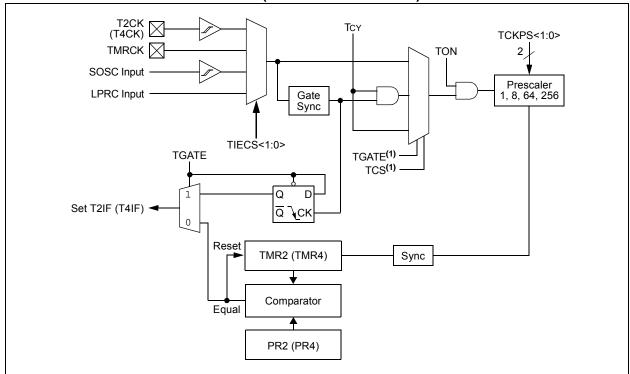
Note 1: The timer clock input must be assigned to an available RPn/RPIn pin before use. See Section 11.4 "Peripheral Pin Select (PPS)" for more information.
