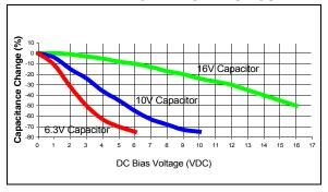
When selecting a ceramic capacitor to be used with the internal voltage regulator, it is suggested to select a high-voltage rating, so that the operating voltage is a small percentage of the maximum rated capacitor voltage. The minimum DC rating for the ceramic capacitor on VCAP is 16V. Suggested capacitors are shown in Table 2-1.
