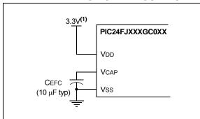
Note 1: This is a typical operating voltage. Refer to Section 37.0 "Electrical Characteristics" for the full operating ranges of VDD.
