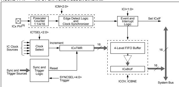
Note 1: The ICx inputs must be assigned to an available RPn/RPIn pin before use. See Section 11.4 "Peripheral Pin Select (PPS)" for more information.
