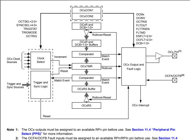
The OCFA/OCFB Fault inputs must be assigned to an available RPn/RPIn pin before use. See Section 11.4
