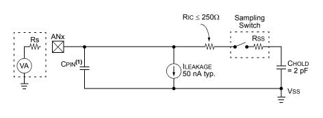
Legend: CIN = Pin Capacitance + Channel MUX Capacitance<sup>(1,2)</sup>
