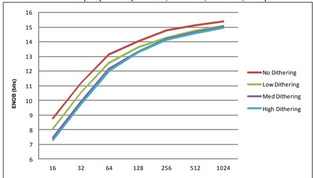
FIGURE 38-4: ENOB (SINAD) vs. OSR (VDD = 3.3V, VREF = 2.0V, Fin = 25 Hz, +25°C)
