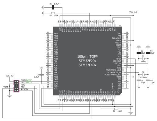
Figure 7-3: Connection schematics for 100-pin STM32F20x/STM32F40x MCU via 2x5 male header
