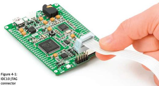
For connection with a target device mikroProg<sup>™</sup> uses IDC10 JTAG connector, as shown on **Figure 4-1**. In order to make proper connection with the target board it is necessary to pay attention to IDC10 connector pinout. Every pin has a different purpose and for easy orientation IDC10 connector is marked with a little knob and incision between pins number 9 and 7, **Figure 5-1**.
