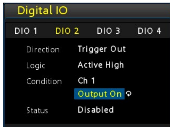
Here, channel 1 of the optional digital I/O interface is used as a trigger input.
