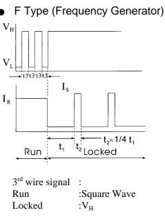
t<sub>3</sub>:F Type has open collector circuit designed for rpm measurement.
