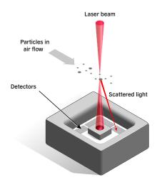
mine the size distribution and mass concentration of the particles. With an integrated ASIC, no external processing is needed, and the SPS6x provides fully processed values through an I<sup>2</sup>C communication.
