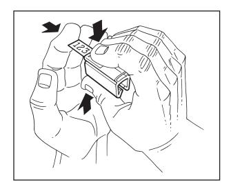
PTC is advantageous in applications where a fast mounting of holder and marker tag is desired. Irrespectable of electrical connection of cable or wire being made before or after mounting of the holder. And at the same time when an easy flexible printout on site with alternative solutions are preferred.
