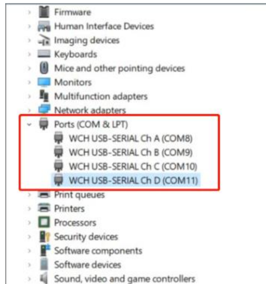
Figure 9: USB-to-UART Interface Displayed on PC
