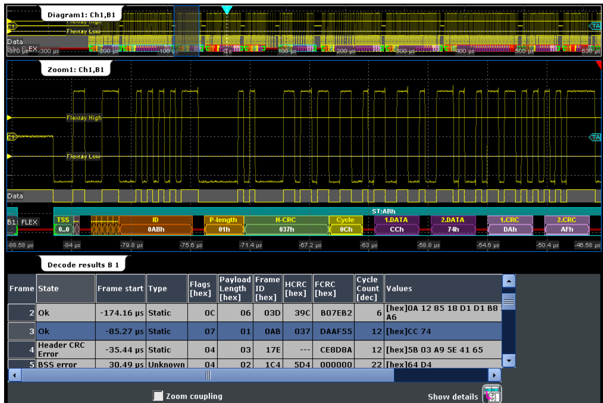
Figure 12-37: FlexRay - decoded dynamic slot and results table
