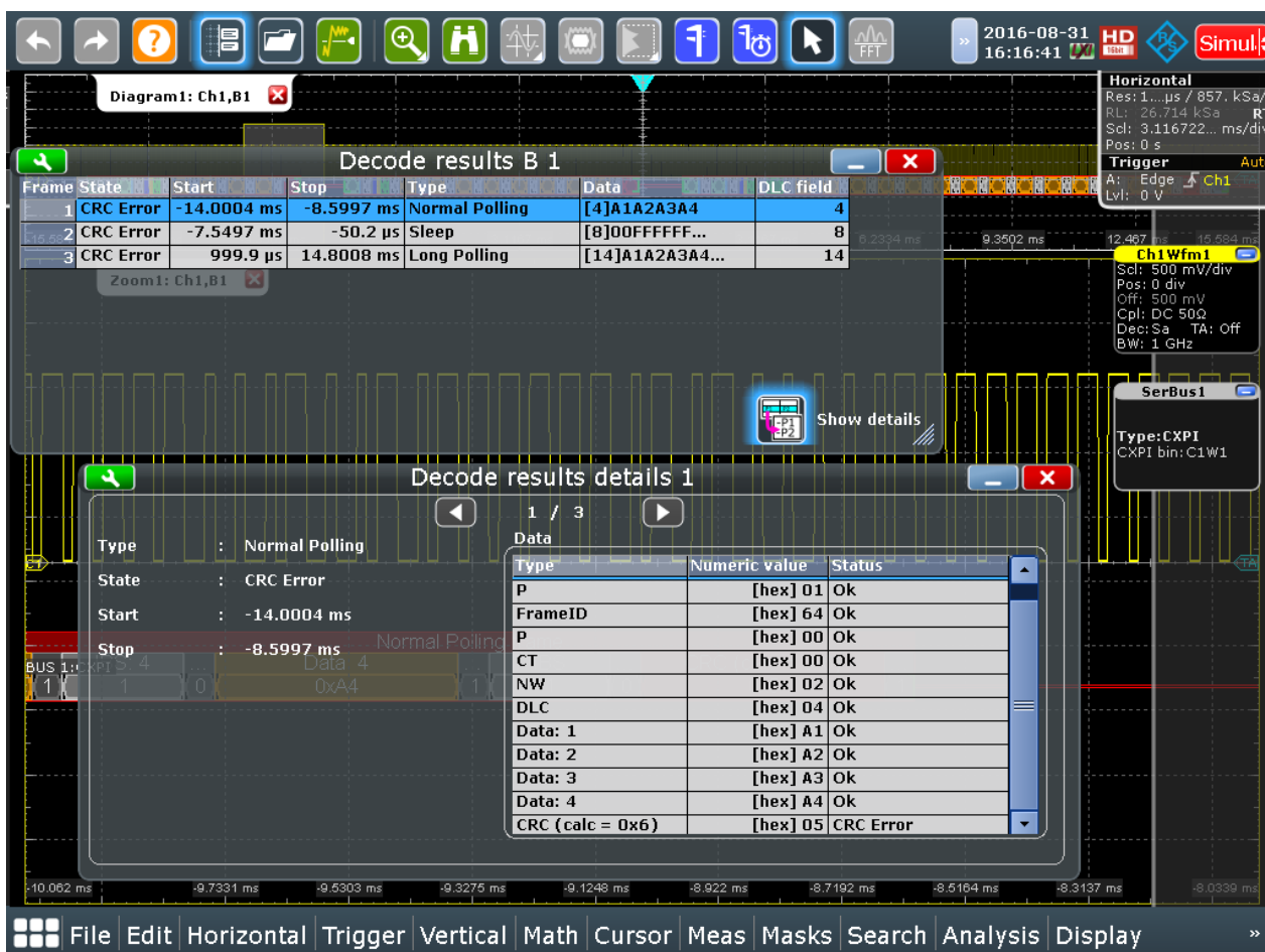
Figure 12-123: Decoded CXPI signal result tables, normal polling frame with CRC error
