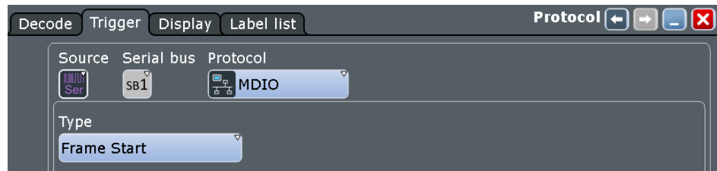
Figure 12-95: MDIO trigger event settings dialog
