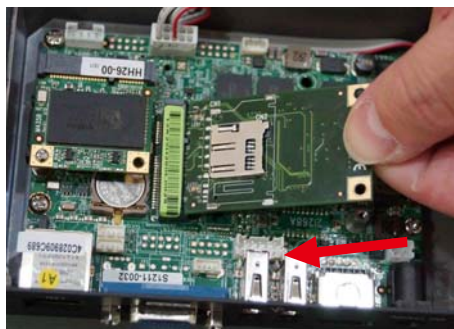
6. Install the full size MINI PCI-E card at the angle of 45°. (Such as 3G card module, Wireless card module or GPS card module)
