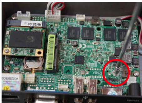
5. Unfasten the round-headed M2*6 screw for the full size MINI PCI-E.
