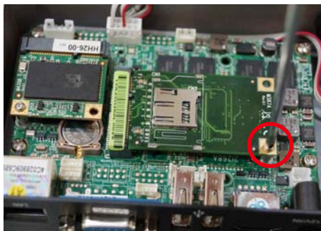
8. Fasten round-headed M2*6 screw.
