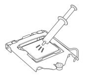
**CAUTION!** Apply the Thermal Interface Material to the CPU heatsink and CPU before you install the heatsink and fan if necessary.
