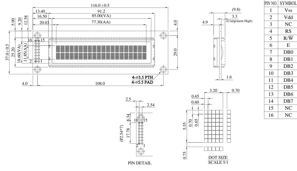
The non-specified tolerance of dimension is  $\pm 0.3 \mbox{ mm}$  .
