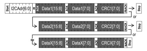
Dark areas with white text indicate that the sensor controls the SDA (Data) line.
