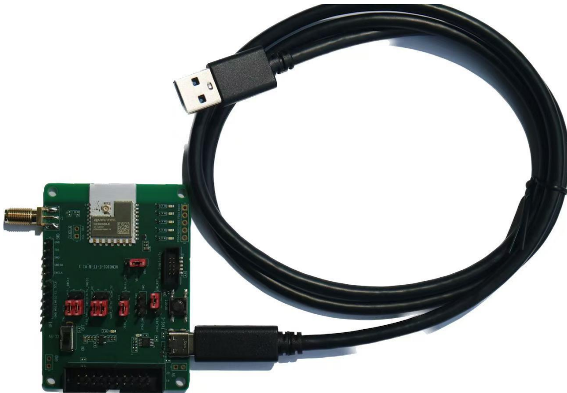
Figure 4: TE-B Kit Assembly
