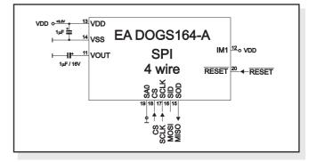
To guarantee an error-free functionality and initialization of display it is recommended to operate the reset input actively. This can be done via microcontroller port or external circuit. Here's an application example:
