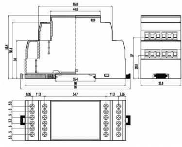
The CEM35 electronic housing is realized for connections up to 24 poles.
