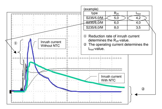
Fig.3 Typical current characteristic in load after turning on
