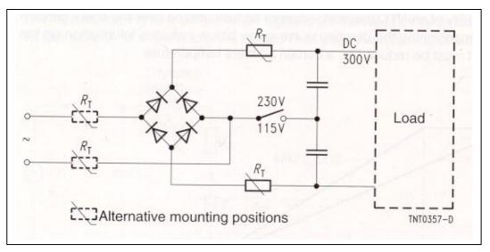
Fig.2 Possible locations of NTC for inrush current limiting
