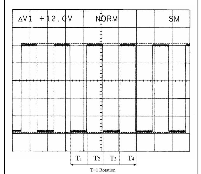
T=T1+T2+T3+T4 = (1 Rotation)  $T1=T2=T3=T4= \frac{60}{4 \times \text{rpm}}$
