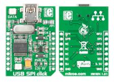
USB SPI Click<sup>™</sup> is an accessory board in **mikroBUS**<sup>™</sup> form factor. It's a compact and easy solution for adding SPI serial communication via USB cable. It features **MCP2210** USB-to-SPI protocol converter with GPIO as well as USB MINI B connector. USB SPI Click<sup>™</sup> communicates with target board via SPI interface as a master device. The board is designed to use 3.3V or 5V power supply. It has a LED diode (GREEN) that indicates the presence of power supply.
