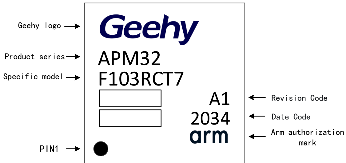
Figure 16 LQFP64-64 pins, 10×10mm package identification
